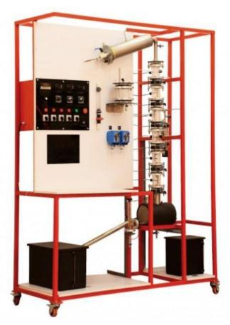
Continuous distillation, a form of distillation, is an ongoing separation in which a mixture is continuously (without interruption) fed into the process and separated fractions are removed continuously as output streams. Distillation is the separation or partial separation of a liquid feed mixture into components or fractions by selective boiling (or evaporation) and condensation. The process produces at least two
