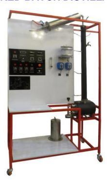
This device is used for familiarizing with the operation of packed bactch distillation columns. With the instrumentation and other equipment installed on the device, the batch distillation process can be extensively investigated.
