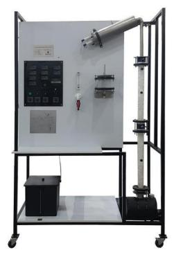
This device is used for familiarizing with the operation of packed bactch distillation columns. With the instrumentation and other equipment installed on the device, the batch distillation process can be extensively investigated.
