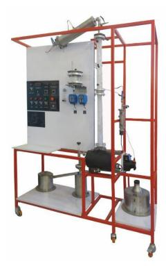
The rectification columns are used for the separation of liquid phases. They operate according to the principle of distillation. Distillation is a separation process that includes the partial evaporation of a liquid phase and the condensation of the resulting gas phase. The separation process of rectification is an energyyefficient distillation process with several stages. The substance mix recommended for the operation of the experimental plant is water-ethanol.
