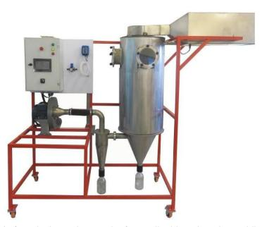
Spray drying is a method of producing a dry powder from a liquid or slurry by rapidly drying with a hot gas. This is the preferred method of drying of many thermally-sensitive materials such as foods and pharmaceuticals.
