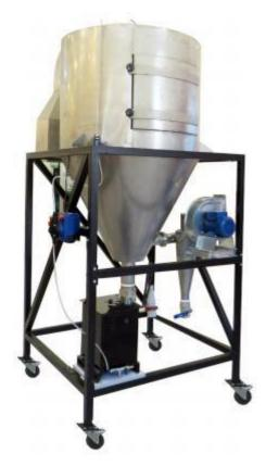
Spray drying is a method of producing a dry powder from a liquid or slurry by rapidly drying with a hot gas. This is the preferred method of drying of many thermally-sensitive materials such as foods and pharmaceuticals.
