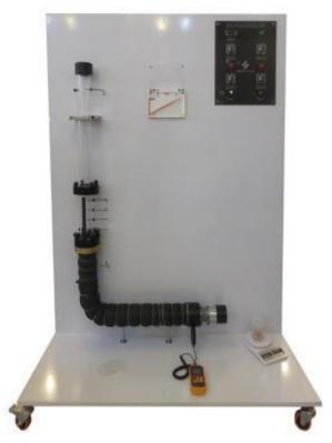
The dryer works by blowing ambient air and passing it through the electric heater, which increases the air temperature is adjusted by changing the voltage. The amount of air and, as a result, the air exit speed
