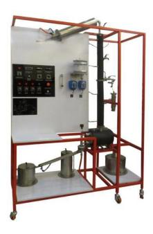
The rectification columns are used for the separation of liquid phases. They operate according to the principle of distillation. Distillation is a separation process that includes the partial evaporation of a liquid phase and the condensation of the resulting gas phase. The separation process of rectification is an energyyefficient distillation process with several stages. The substance mix recommended for the operation of the experimental plant is water-ethanol.
