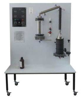
Accurate data of the equilibrium between liquid and vapour for two phases mixture is a vital part of designing of chemical pro-cesses and distillation devices. In this unit we study the liquid-vapor equilibrium of the mixture of ethanol and water the present experiments were conducted at various temperature at 1 atm and the ex-perimental data were collected and some were compared with theorical results.
