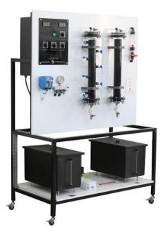
Adsorbtion is the process of disposing of particles dissolved in water using absorbent materials. During this process, various factors affect the absorption of solution, such as temperature, type and diameter of absorbent, pH, etc. In this unit, two glass columns are used. Activated carbon is used as absorbent and methylene blue solution is used as absorbate.
