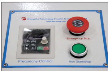
Frequency Converter Control Expected rotate speed can be selected according to experiment need, minimum scale of rotate speed is 0.2 rpm. Frequency converter owns protection device of under voltage and over voltage which provides necessary protection for motor.
