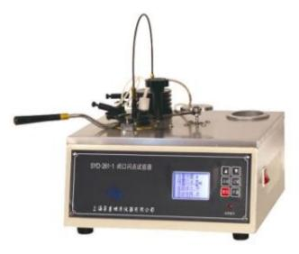
This instrument is designed and manufactured as per standards GB/T 261-2008 Determination of Flash Point - Pensky-Martens closed cup method and ASTM D93 Standard Test Methods for Flash Point by Pensky-Martens Closed Cup Tester. It is used to make determination of the closed cup flash point of the petroleum products.
