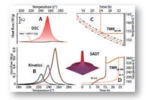
An adiabatic experiment with a Phi factor = 3.2 was performed for the final validation of the simulation, and compared to calculated adiabatic data (D).
