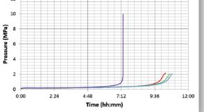
This series of tests has shown the impact of concentration on the temperature and pressure rise of DTBP. A significant increase of concentration leads to drastically higher thermal and pressure risks.
