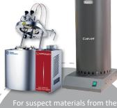
DSC stage and due to the central role of gas releasing reactions in plant process hazards, larger samples of about 5-10g are heated to destruction in cells equipped with a pressure sensor. The focus of the study is to understand volume of gas evolved, when and how fast it's evolved in order to understand it's decomposition profile.
