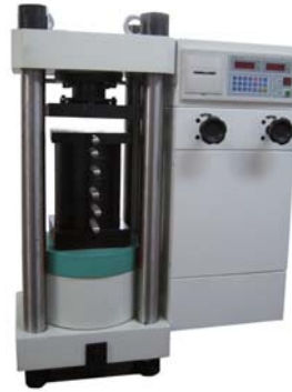
CH42200 Using Space thickness block and upper plate spherical bearing
