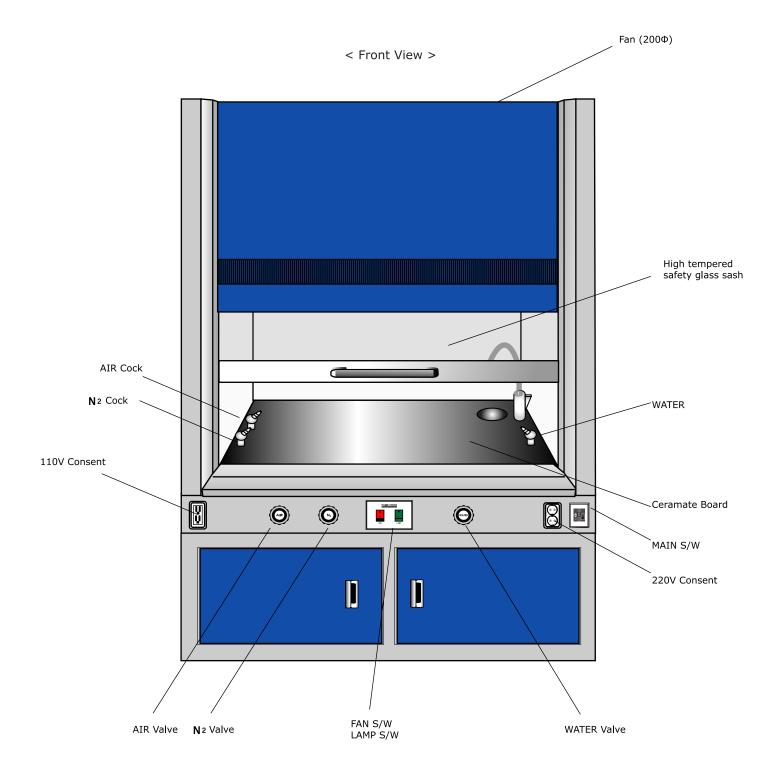
Out size :  $1500 \times 800 \times 2300$  (W x D X H,mm)
